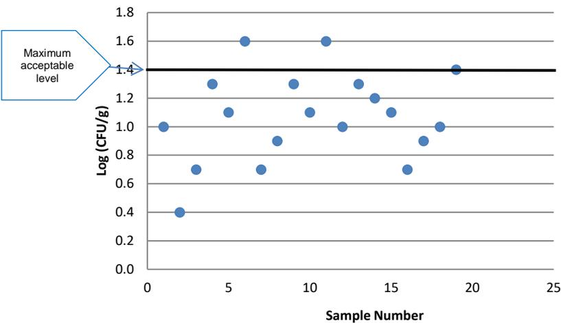
Chart 2 depicts a loss of process control due to excess variability. This is reflected in both an increased number of results above the maximum acceptable level and an increase in the scatter of points below the maximum acceptable level.
