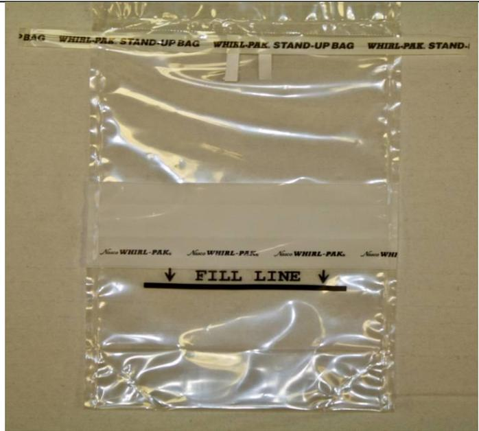
3. Collect sufficient product to fill the two Whirl-Pak® bags up to the fill-line on the bag.
