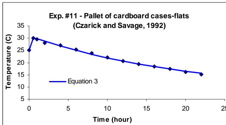
FIGURE D7 OBSERVED AND PREDICTED TEMPERATURES VERSUS TIME FOR AVAILABLE EXPERIMENTAL DATA: PALLET OF CARDBOARD CASES—FLAT—EXPERIMENT #11.<sup>1</sup>
