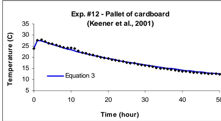
FIGURE D8 OBSERVED AND PREDICTED TEMPERATURES VERSUS TIME FOR AVAILABLE EXPERIMENTAL DATA: PALLET OF CARDBOARD—EXPERIMENT #12.<sup>5</sup>
