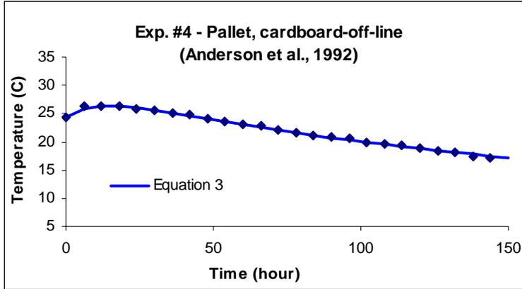
FIGURE D4 OBSERVED AND PREDICTED TEMPERATURES VERSUS TIME FOR AVAILABLE EXPERIMENTAL DATA: PALLET, CARDBOARD OFF-LINE—EXPERIMENT #4.<sup>3</sup>
