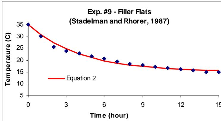
FIGURE D6 OBSERVED AND PREDICTED TEMPERATURES VERSUS TIME FOR AVAILABLE EXPERIMENTAL DATA: FILLER FLATS—EXPERIMENT #9.<sup>4</sup>
