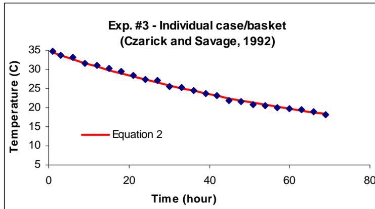
FIGURE D3 OBSERVED AND PREDICTED TEMPERATURES VERSUS TIME FOR AVAILABLE EXPERIMENTAL DATA: INDIVIDUAL CASE/BASKET—EXPERIMENT #3.<sup>1</sup>
