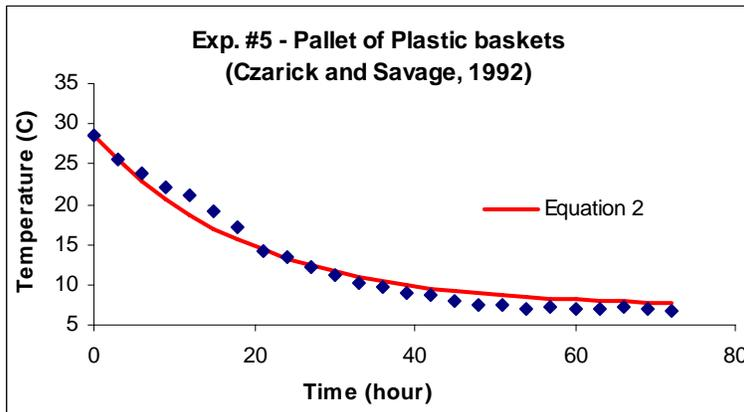
FIGURE D5 OBSERVED AND PREDICTED TEMPERATURES VERSUS TIME FOR AVAILABLE EXPERIMENTAL DATA: PALLET OF PLASTIC BASKETS—EXPERIMENT #5.<sup>1</sup>
