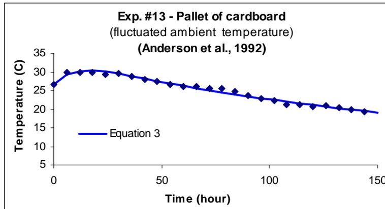
FIGURE D9 OBSERVED AND PREDICTED TEMPERATURES VERSUS TIME FOR AVAILABLE EXPERIMENTAL DATA: PALLET OF CARDBOARD—EXPERIMENT #13.<sup>3</sup>
