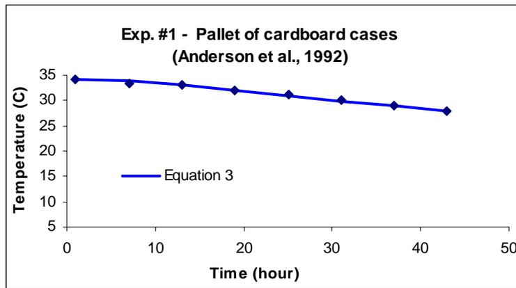
FIGURE D1 OBSERVED AND PREDICTED TEMPERATURES VERSUS TIME FOR AVAILABLE EXPERIMENTAL DATA: PALLET OF CARDBOARD CASES—EXPERIMENT #1.<sup>3</sup>
