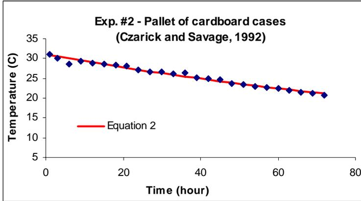
FIGURE D2 OBSERVED AND PREDICTED TEMPERATURES VERSUS TIME FOR AVAILABLE EXPERIMENTAL DATA: PALLET OF CARDBOARD CASES—EXPERIMENT #2.<sup>1</sup>
