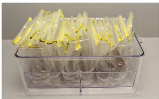
1c. Adding up to 32 samples per container; it's optional to use a secondary bag to hold samples.
