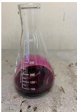
Figure 6: Digested sample with initial addition potassium permanganate ( \text{KMnO}_4 ). Photo courtesy of Bruno Giri, USDA-FSIS
