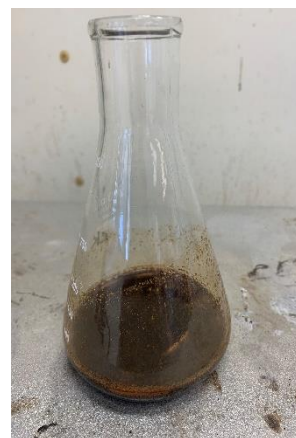
Figure 7: Digested sample with the addition of potassium permanganate ( \text{KMnO}_4 ) and boiled for several minutes. Photo courtesy of Bruno Giri, USDA-FSIS.
