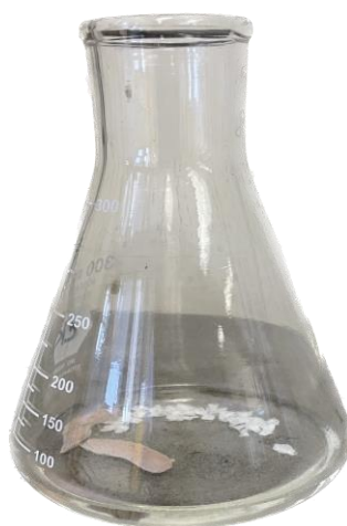
Figure 4: Sample after addition of the silver nitrate ( \text{AgNO}_3 ) and nitric acid ( \text{HNO}_3 ). Photo courtesy of Bruno Giri, USDA-FSIS
