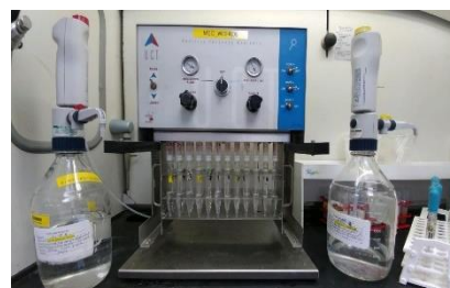
Figure 14: Samples undergoing SPE cleanup for GC-MS/MS Analysis. Photo courtesy of Ryan Matsuda USDA-FSIS
