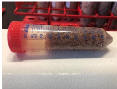
Figure 8: Samples with QuEChERS salts. Photo courtesy of Jason Stone USDA-FSIS
