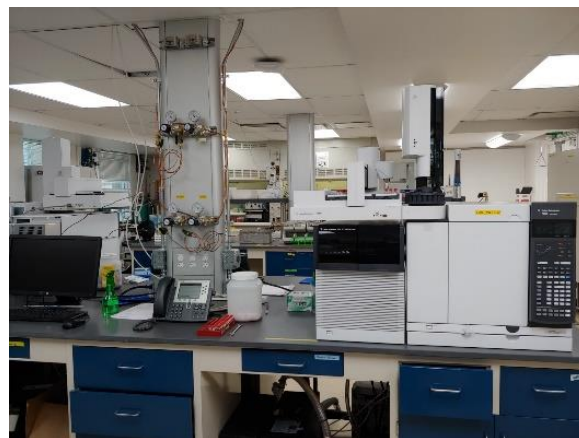
Figure 17: Example of a GC-MS/MS instrument. Photo courtesy of Ryan Matsuda USDA-FSIS
