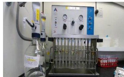
Figure 11: Solid phase extraction manifold. Photo courtesy of Ryan Matsuda USDA-FSIS
