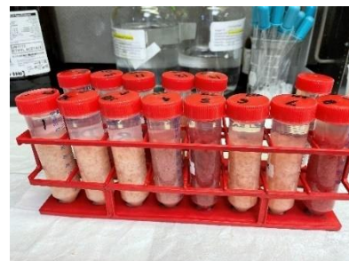
Figure 6: Ethyl acetate added to controls and samples. Photo courtesy of Ryan Matsuda, USDA-FSIS
