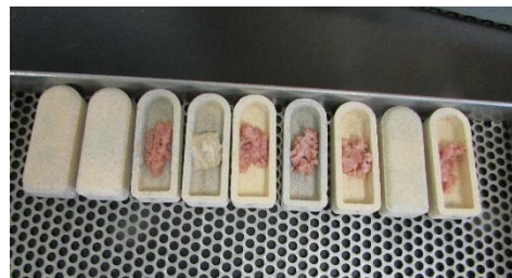
Figure 4: Samples in ceramic boat before analysis. Photo courtesy of Killani Kadri, USDA-FSIS
