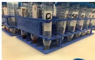
Figure 5: Plasma samples equilibrate at room temperature. Photo courtesy of Noelle Lebow, USDA-FSIS
