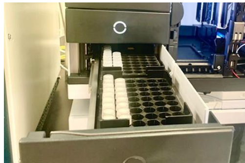
Figure 11: Prepared samples in UHPLC-MS-MS instrument. Photo courtesy of Qing Delgado, USDA-FSIS
