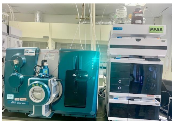
Figure 12: 1290 Infinity UHPLC with Sciex QTrap 6500+ mass spectrometer. Photo courtesy of Qing Delgado, USDA FSIS.
