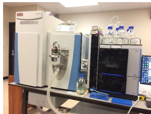
Figure 5: Example of HRAM LC-MS instrument with high resolution. Photo courtesy of Abdulahi Duale, USDA-FSIS
