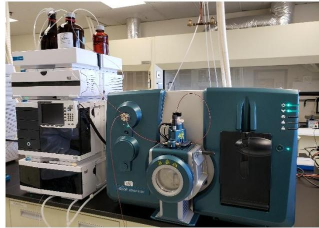
Figure 6: 1290 Infinity UHPLC with Sciex QTrap 6500+ mass spectrometer. Photo courtesy of Sam Zipperer, USDA FSIS.
