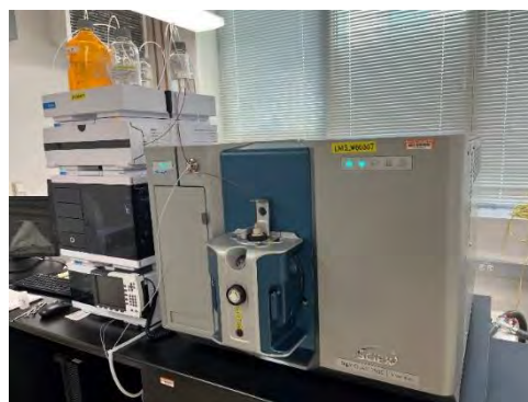
Figure 9: 1290 Infinity UHPLC with SCIEX 7500 QTrap Activated mass spectrometer. Photo courtesy of Stephen Kubota, USDA-FSIS.
