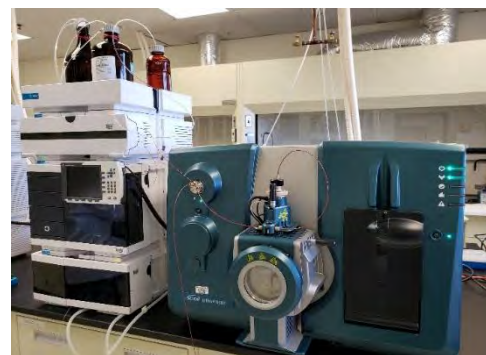
Figure 8: 1290 Infinity UHPLC with SCIEX QTrap 6500+ mass spectrometer. Photo courtesy of Sam Zipperer, USDA-FSIS.
