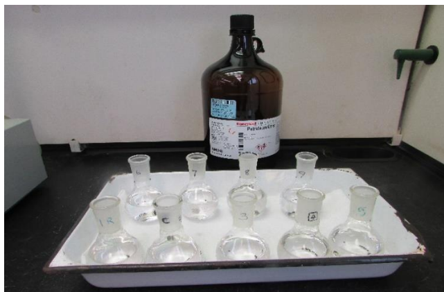
Figure 9: Extraction flasks, boiling chips and petroleum ether. Photo courtesy of Killani Kadri, USDA FSIS
