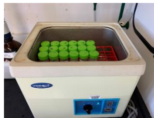
Figure 7: Immerse tubes into an ultrasonic bath. Photos courtesy of Bruno Giri, USDA-FSIS
