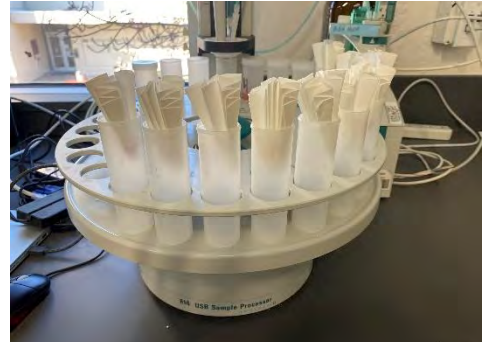
Figure 6: Samples undergoing filtration and titration. Photo courtesy of Ryan Matsuda, USDA-FSIS
