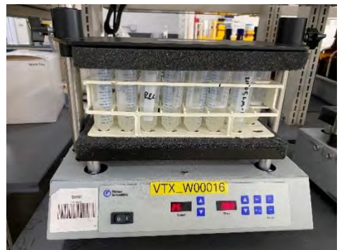
Figure 7: Clean up through dispersion SPE. Photo courtesy of Ryan Matsuda, USDA-FSIS
