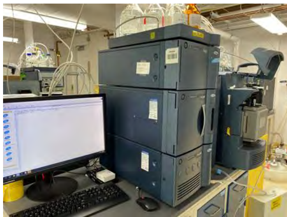
Figure 10: LC-MS-MS instrument. Photo courtesy of Ryan Matsuda, USDA-FSIS
