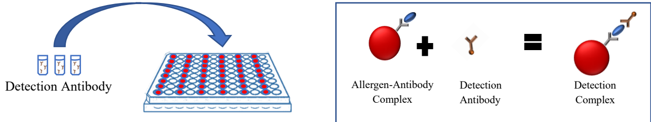
Figure 7: Transfer detection antibody to wells and incubate. Figure courtesy of Marie Kelleher, USDA-FSIS
