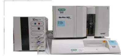
Figure 9: Fluorescence plate reader. Photo courtesy of Marie Kelleher, USDA-FSIS
