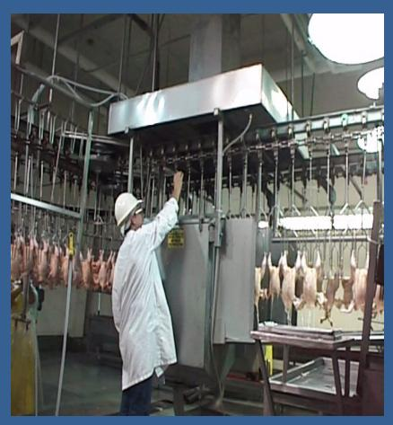
Point in the slaughter process where contaminated eviscerated carcasses are reprocessed on-line following the provisions of a waiver granted in accordance with 9 CFR 381.3(b)
