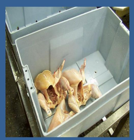
Point in slaughter and further processing where contaminated eviscerated carcasses & parts that have fallen on the floor, or otherwise have become contaminated off-line, are reconditioned in order to restore sanitary conditions.
