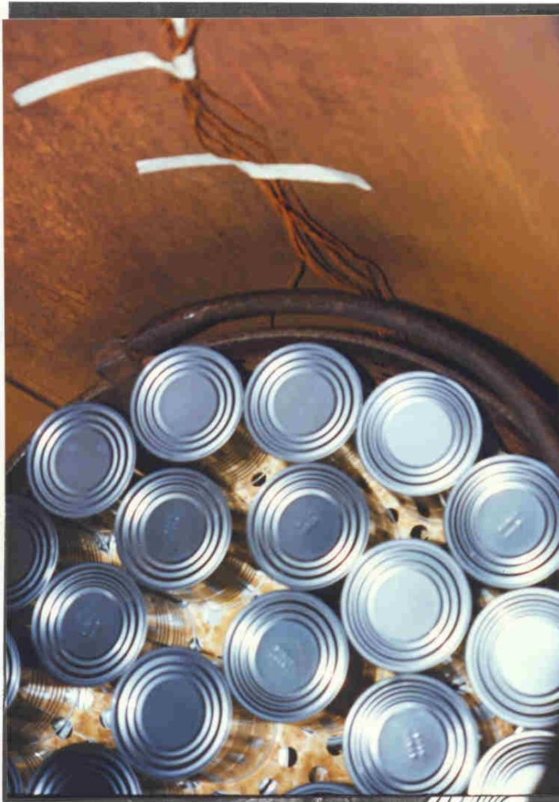
Thermocouple leads must be placed so they are not damaged during the test
