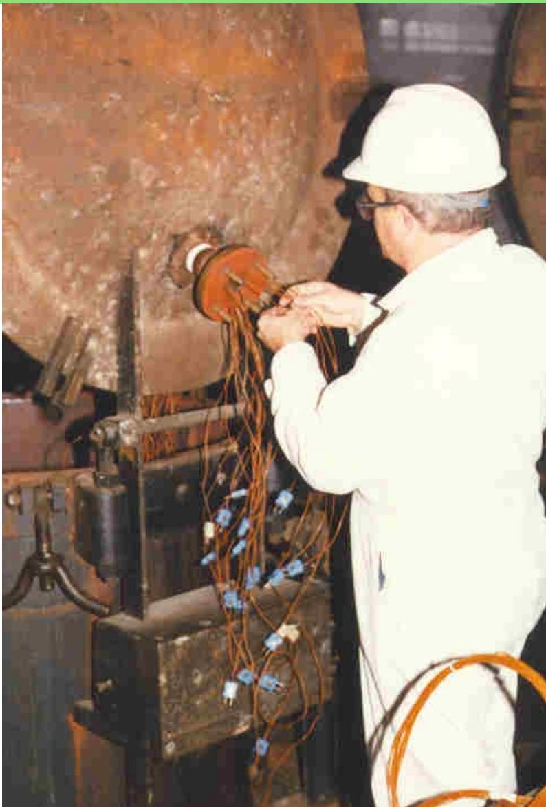
Thermocouple wires (leads) are fed into retort through steam tight gasket.
