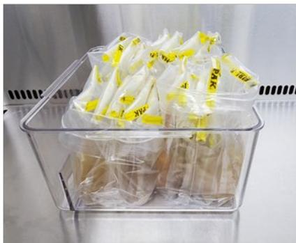
1c. Adding up to 32 samples per container; it's optional to use a secondary bag to hold samples.
