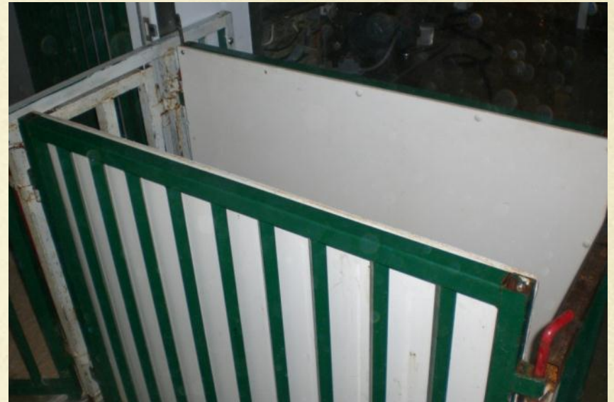
Plastic lining in stun box area to insulate electrical current
