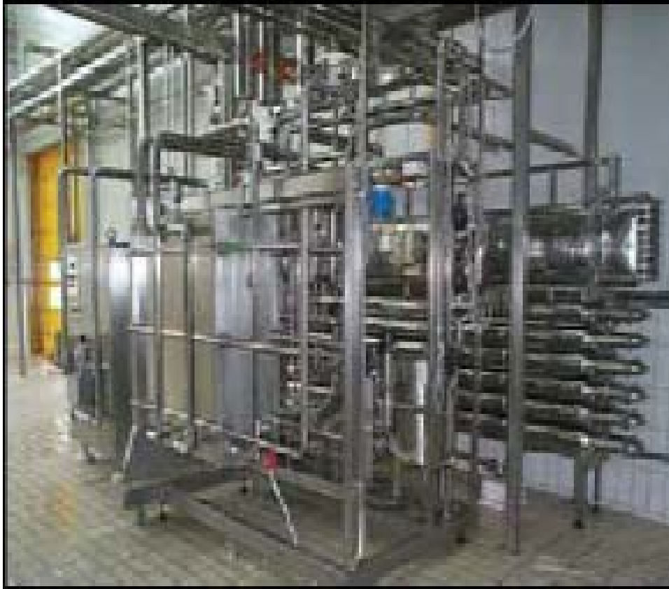
Figure 1 – Pasteurizer with tubular heat exchanger and plate heat exchanger
