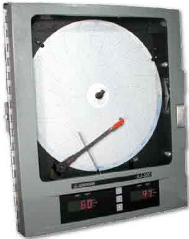
**The temperature/time recorder should agree as close as possible with MIG/RTD but never higher-** Accuracy to 1°F-Pen arc adjusted properly-Time of day set properly-Prevent unauthorized changes with a lock or notice.
