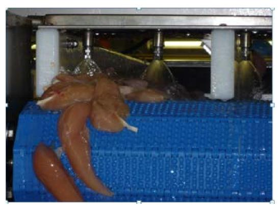
This image also shows incomplete coverage. In particular, no spray is applied to the underside of products. In addition, not all pieces on the conveyor belt are being treated because the arc of the spray is too narrow to cover all product that could pass on the conveyor. The spray is also not being applied to all pieces due to product piling up and overlapping on the conveyor belt.
