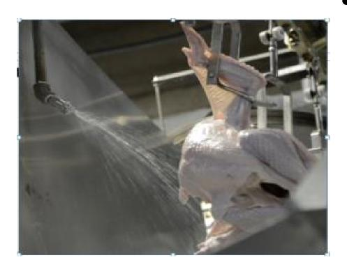
This image shows incomplete coverage. In particular, only part of the carcass is receiving the spray. If complete coverage can't be achieved then the intervention will not be as effective.
