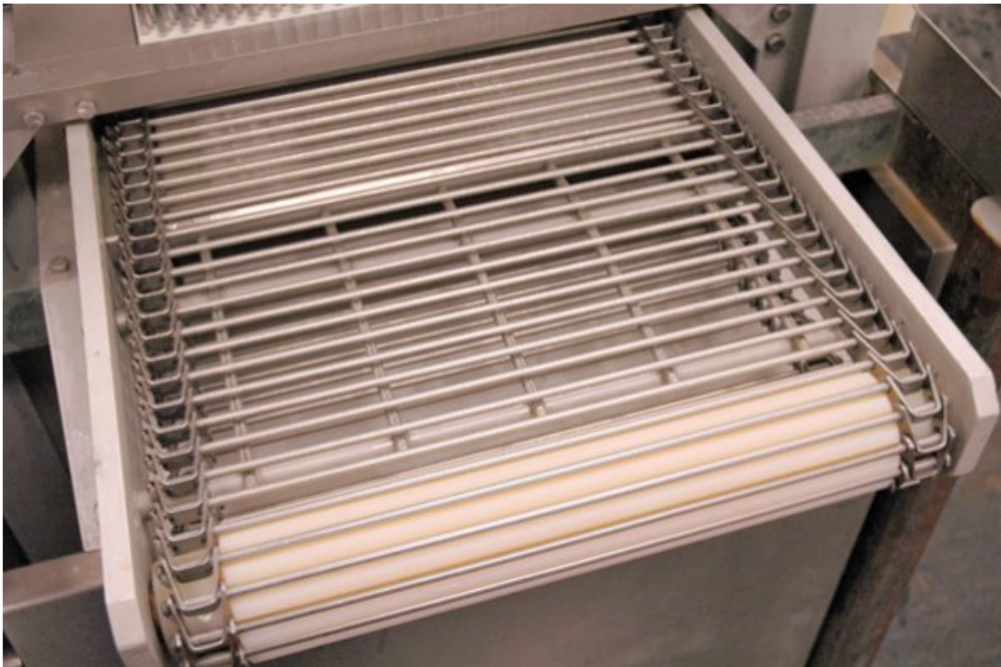
A conveyor belt with a hollow roller under the belt. Lm could be harbored in the hollow roller and spread to the belt.
